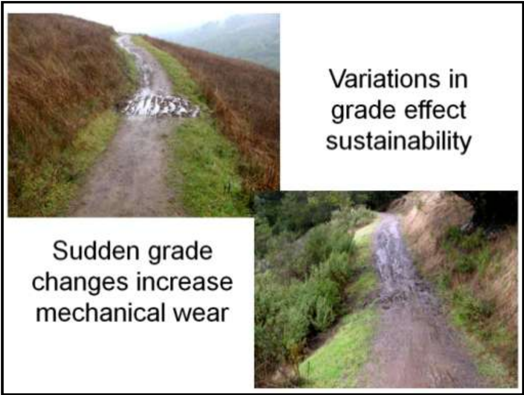
Figure #12 Abrupt Grade Changes
